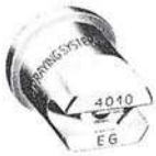
EG Tip Type EG spray tips produce a uniform spray distribution of medium sized droplets. The spray tip orifice is precision machined to accurately control flow rates.
